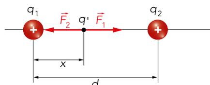
$$|F_1| = |F_2| \rightarrow K_0 \cdot \frac{q_1 \cdot q'}{x^2} = K_0 \cdot \frac{q_2 \cdot q'}{(d-x)^2} \rightarrow \frac{q_1}{x^2} = \frac{q_2}{(d-x)^2} \rightarrow (q_1 - q_2) \cdot x^2 - 2 \cdot d \cdot q_1 \cdot x + q_1 \cdot d^2 = 0$$
