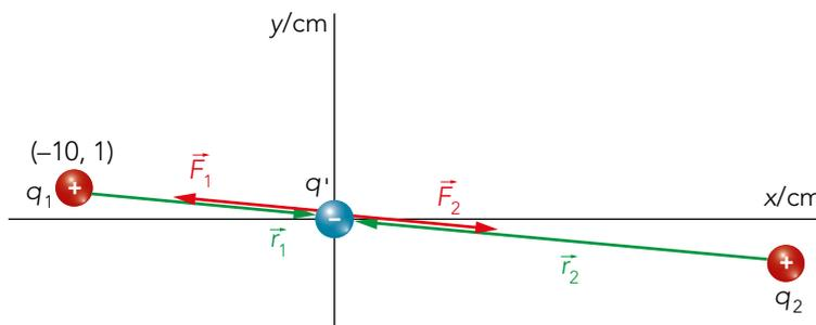
$$|F_1| = |F_2| \rightarrow K_0 \cdot \frac{q_1 \cdot |q'|}{r_1^2} = K_0 \cdot \frac{q_2 \cdot |q'|}{r_2^2} \rightarrow \frac{q_1}{r_1^2} = \frac{q_2}{r_2^2} \rightarrow r_2 = \sqrt{\frac{q_2}{q_1}} \cdot r_1 = \sqrt{\frac{9}{3}} \cdot \sqrt{10^2 + (-1)^2} \approx 17,4 \text{ cm}$$
