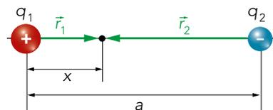
$$V = V_1 + V_2 = K_0 \cdot \frac{q_1}{r_1} + K_0 \cdot \frac{q_2}{r_2} = K_0 \cdot \frac{q_1}{x} + K_0 \cdot \frac{q_2}{a-x} = 0 \rightarrow \frac{q_1}{x} = -\frac{q_2}{a-x} \rightarrow q_1 \cdot (a-x) = -q_2 \cdot x$$
