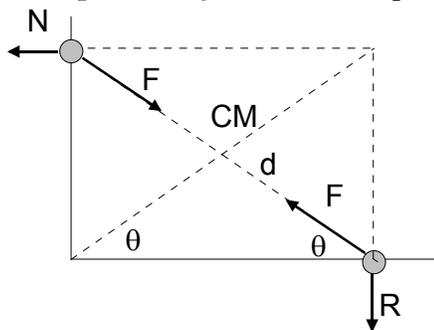
$$\begin{aligned} m\ddot{x} &= -F \cos \theta = -\frac{k}{d^2} \cos \theta = -\frac{k}{d^3} x \\ m\ddot{y} &= -F \sin \theta = -\frac{k}{d^2} \sin \theta = -\frac{k}{d^3} y \end{aligned}$$
