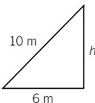
$$\begin{aligned} 10^2 &= h^2 + 6^2 \rightarrow h^2 = 100 - 36 = 64 \rightarrow \\ &\rightarrow h = 8 \text{ m} \end{aligned}$$
