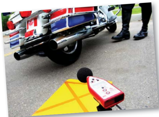
Device used to measure motorcycle noise levels
